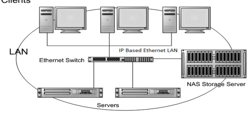
NAS is storage that is connected directly to a network, such as a LAN, that provides file-level access to data using standard protocols such as NFS (Network File System) or CIFS (Common Internet File System).
