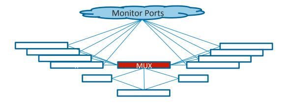
Aggregates all filter switches in a data center Directs traffic to either service nodes or delivery interfaces
