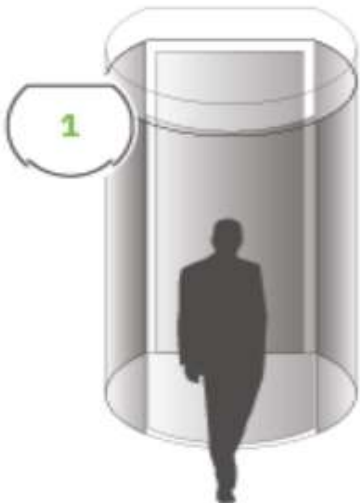
TAILGATING : IN OPPOSITE DIRECTION DETECTION VIA: CONTACT MAT
