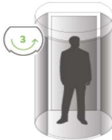
TAILGATING : IN SAME DIRECTION DETECTION VIA: CONTACT MAT
