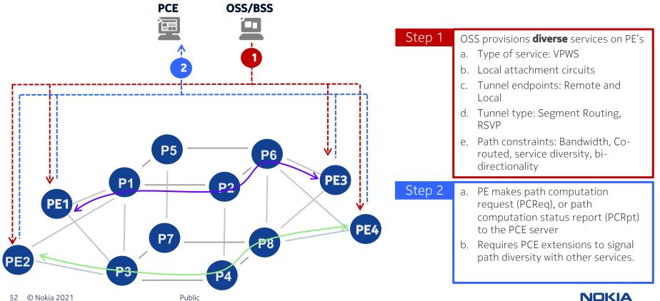
Use case 8: Service creation with a path computation element (PCE) (cont.) Co-routed service node provisioning
