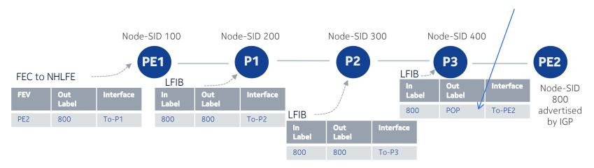
PHP based on p-bit setting of Prefix-SID advertised by PE2
