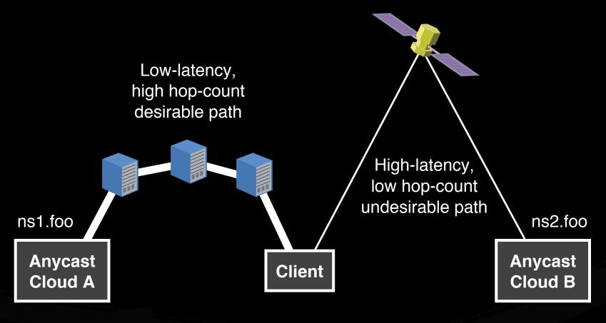
Split the anycast deployment into "clouds" of locations, each cloud using a different IP address and different routing policies.
