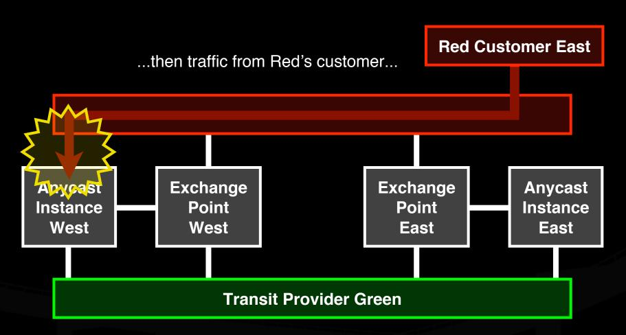
...will be misdelivered to the remote anycast instance, because a customer connection...
