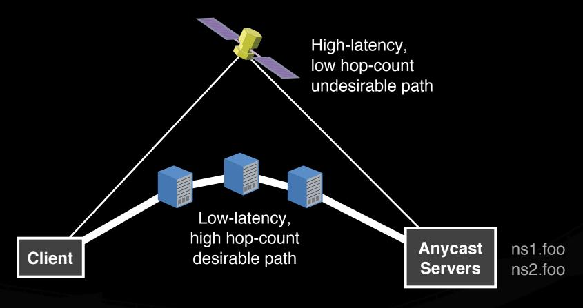
The resolver uses different IP addresses for its fail-over mechanism, while anycast uses the same IP addresses.
