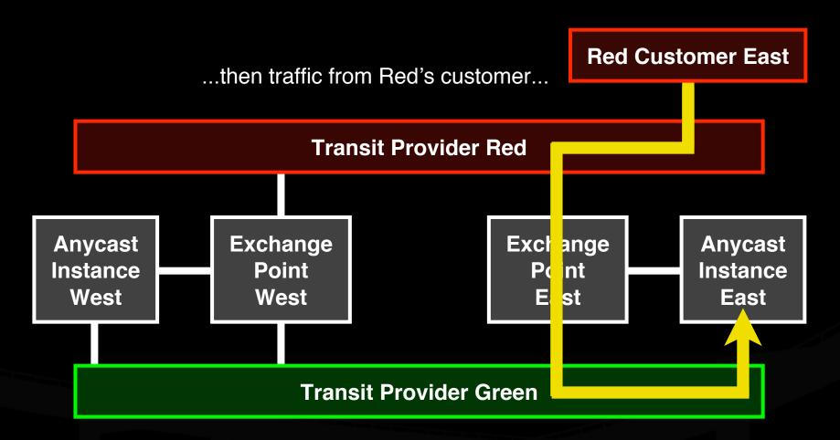
...is delivered from Red to Green via local peering, and reaches the local anycast instance.
