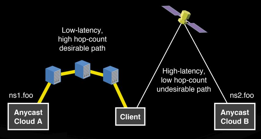
This allows anycast to present the nearest servers, and allows the resolver to choose the one which performs best.
